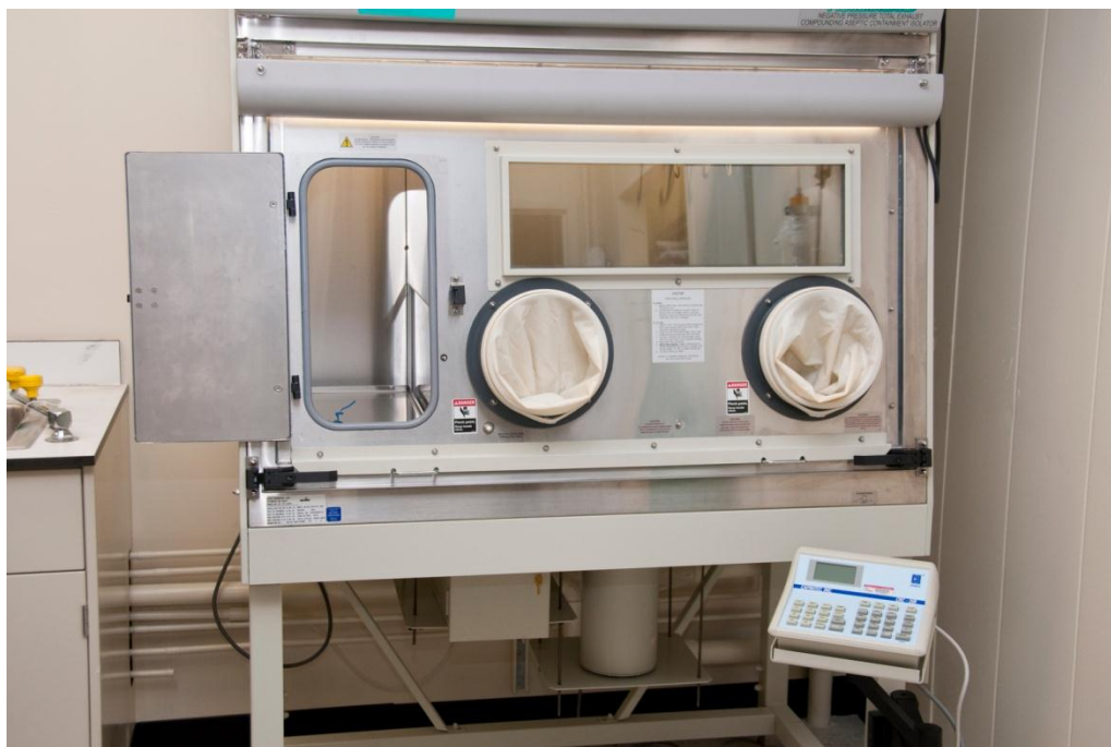
Figure 7-8. ISO Class 5 Lead Shielded Cabinet Where 89 Zr-panitumumab Will Be Synthesized
