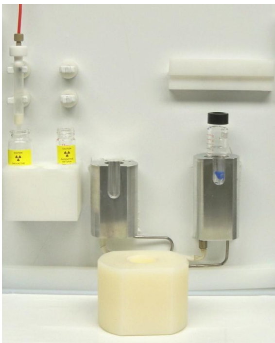
Figure 7-10. ^{89}\text{Zr} Purification Set-Up to Produce Pure ^{89}\text{Zr} -oxalate
