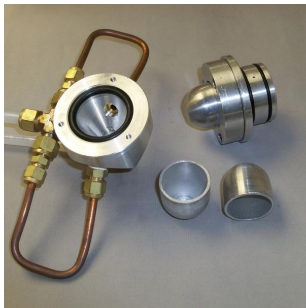
Figure 7-9. GE PETtrace Solid Target Cup Components Used in 89 Zr production
